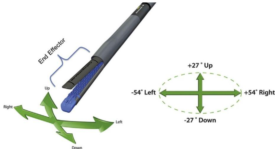
Elliptical range of motion for the robotic stapler.
